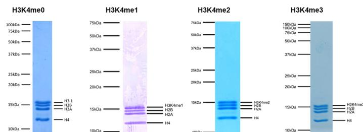
**Protein Gel Data:** Representative Coomassie stained PAGE gel of SNAP-ChIP K-MetStat nucleosomes (2  $\mu$ g each; H3K4me0 = unmodified) demonstrates the purity of histones in the preparation. Sizes of molecular weight markers and positions of the core histones (H2A, H2B, H3 and H4) are indicated. Comparable experiments were performed for the entire K-MetStat Panel. For more information email [techsupport@epicypher.com](mailto:techsupport@epicypher.com).
