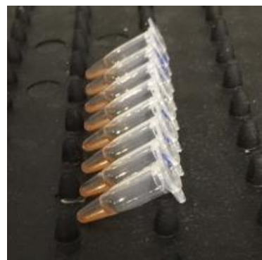
Figure 2. Ensure tube caps are elevated during incubation steps on tube nutator to keep beads in solution.
