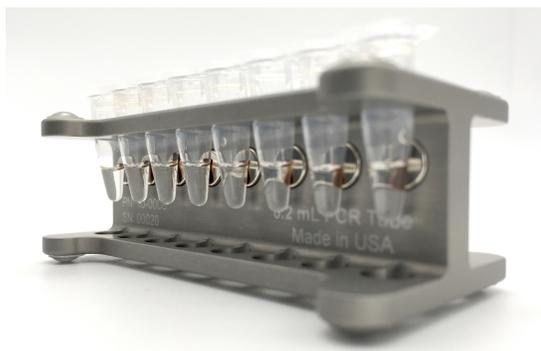
**FIGURE 2 CUTANA™ CUT&RUN 8-strip 0.2mL tubes.** 8-strip 0.2 mL tubes are compatible with the Magnetic Separation Rack (EpiCypher 10-0008) for use during all bead separation steps in the CUT&RUN procedure, including sample immobilization with ConA beads and library preparation. Magnetic Separation Rack is not included in the purchase of this product.
