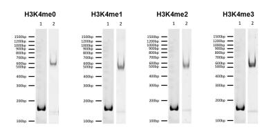
**DNA Gel Data:** Representative images for SNAP-ChIP K-MetStat nucleosomes (H3K4me0 = unmodified) resolved by native PAGE and stained with ethidium bromide to confirm intact nucleosome assembly with minimal free DNA. Lane 1: Free 147 bp DNA used in nuclesome assembly (100 ng). Lane 2: Intact nucleosomes (200 ng). Comparable experiments were performed for the entire K-MetStat Panel. Email <u>techsupport@epicypher.com</u> for more information.
