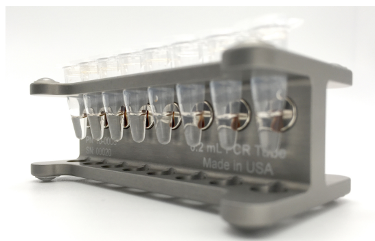
FIGURE 2 Magnetic Separation Rack, oblique view. Rack shown with PCR strip tubes and paramagnetic beads. Note that the 50 - 200 \mu L configuration is being used, and that the magnets are sorting the beads to the side of the tubes.
