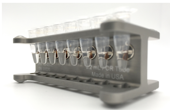
FIGURE 2 Magnetic Separation Rack, oblique view. Rack shown with PCR strip tubes and paramagnetic beads. Note that the 50 - 200 µL configuration is being used, and that the magnets are sorting the beads to the side of the tubes.
