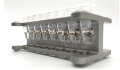
Figure 3: For processing individual samples, it is recommended to multi-channel pipette using 8-strip PCR tubes and compatible magnetic rack (e.g. EpiCypher 10-0008, pictured), increasing experimental throughput and reproducibility.
