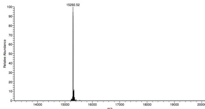
**Mass Spec Data:** Synthetic H3K18cr histone analyzed by high resolution mass spectrometry. Expected mass = 15,291.8 Da. Determined mass = 15,292.5 Da.
