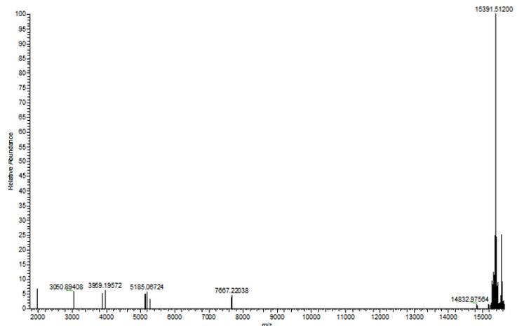
**Mass Spec Data:** H3K4me3, K9,14,18ac protein analyzed by high resolution mass spectrometry. Expected mass = 15,389.8 Da. Determined mass = 15,391.5 Da.
