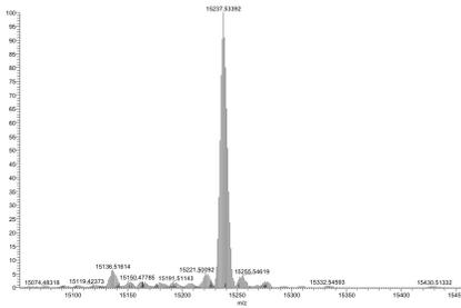
**FIGURE 2 Mass spec data.** Synthetic H3K4me1 histone analyzed by high resolution mass spectrometry. Expected mass = 15,238 Da. Determined mass = 15,237.5 Da.
