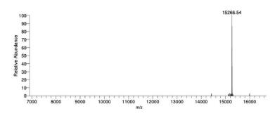
**Mass Spec Data:** Semi-synthetic H3K14ac histone analyzed by high resolution mass spectrometry. Expected mass = 15,266.8 Da. Determined mass = 15,266.54 Da.
