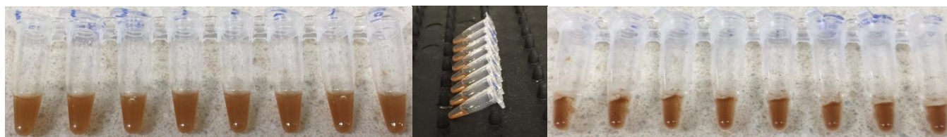
Bead slurry before O/N incubation at 4°C | Nutator O/N | Bead slurry after O/N incubation at 4°C
